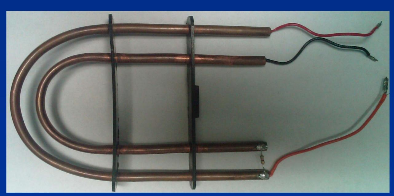
**Figure 2** – TDR Sensor Probe
